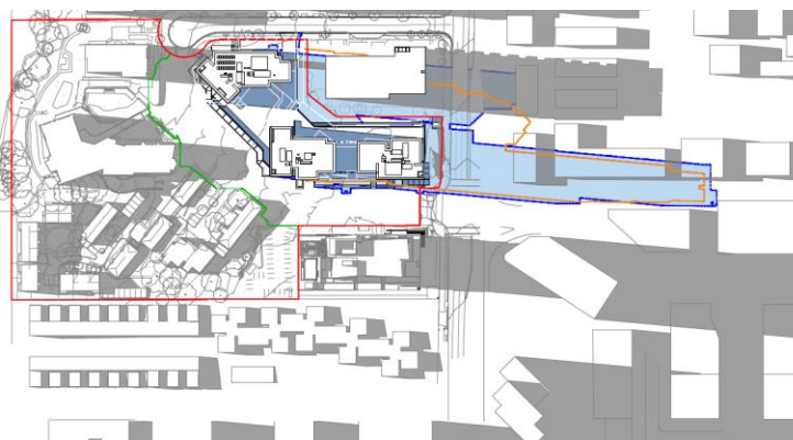
Figure 47 – Shadows cast (in blue) at 3.00pm on 21 June. Source: Plan DA-AR-790-004 as prepared by Turner Studio.
